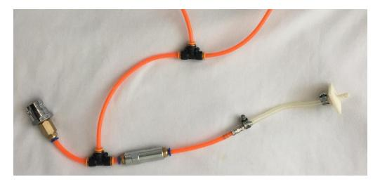
• In the next step, we want to prepare the part related to the pressure gauge. Like the quick connector sector, we need a couple of couplings and a 3.4 to 6mm adaptor
