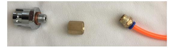
In the next step, take a [RS PRO Tee Tube-to-Tube Adaptor Push in 6 mm, Push in 6 mm to Push in 6 mm, Tube-to-Tube Connection] and Connect two 6 mm hoses to the previous two structures and add a 20 cm hose to the last slot.
