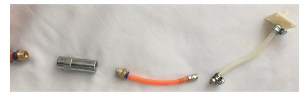
• In the next step, pick the Ohmeda Oxygen Quick-Connecter. For this part You will need to attach a female double head coupling to install a 6 mm hose converter and conduct oxygen.
