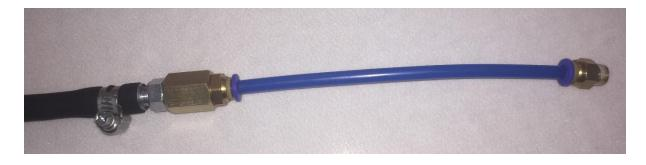
• Cut two pieces of 15 cm ligris hose and place a 1/16 elbow on one side and a 1/8 elbow on the other side.
