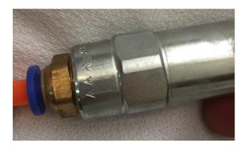
After connecting these items to the check valve You have to take the 3 cm hose and insert one side into another [RS PRO Straight Threaded Adaptor, R 3/4 male to Push in 6 mm, Threaded-to-Tube Connection]
