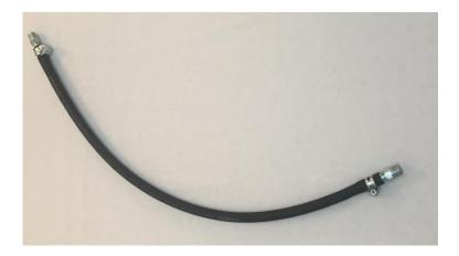
• At this stage, cut 15 cm of 8 mm polyurethane hose and connect an 8 mm to 1/8-inch converter to one end and an 8 mm to 3.4-inch converter to the other end.
