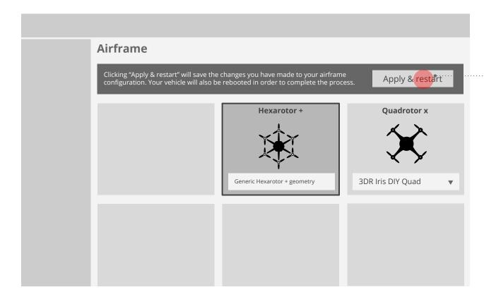
When a different frame type is selected, the button "Apply & restart" appears. The user should tap here to change the configuration
