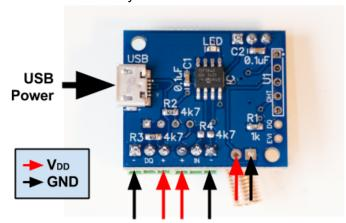
The most convenient way is through the micro USB port. An alternative way is to solder cables to the soldering points to the right of the screw terminals. A third option is to use any of the screw terminal points.
