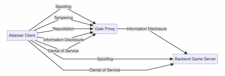
The threat model diagram helps visualize the potential threats identified using the STRIDE methodology. It can show where in the system these threats could occur and the flow of potential attacks.
