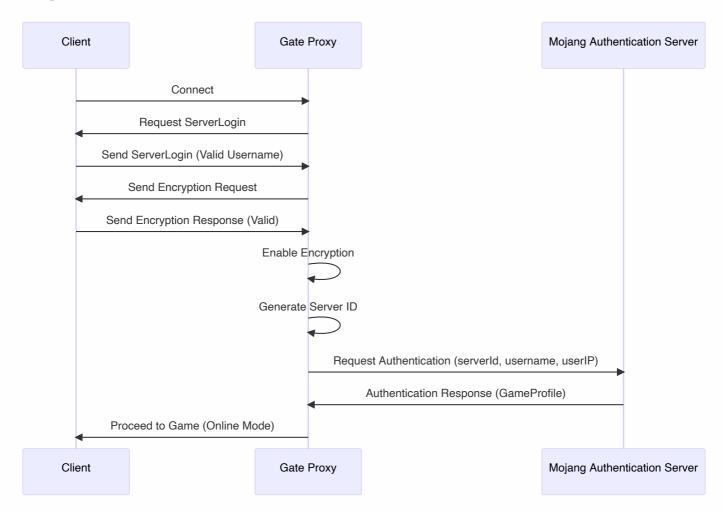
The sequence diagram shows the best-case scenario for the online mode authentication flow. It can help in understanding the order of operations and the exchange of information between the client, proxy, and authentication server.
