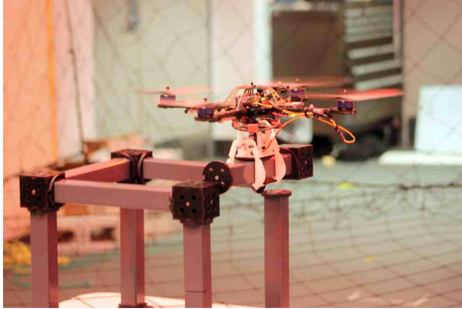
Figure 4.1: Quadrotor assembling part on a cubic structure.
