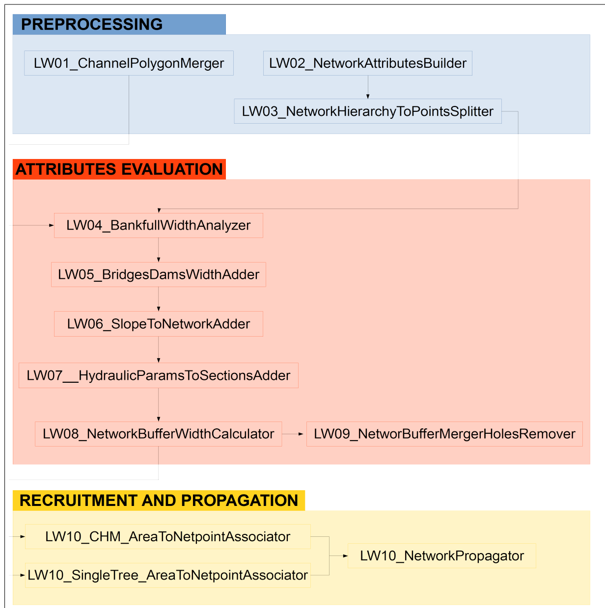
Figure 2.1: Work-flow of the tools for the evaluation of Large Wood recruitment and propagation.
