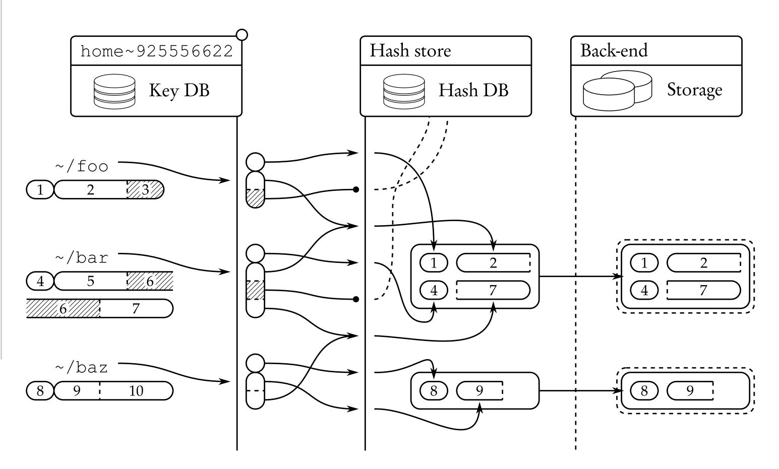
The internals of Hindsight: On the left are the files being backed up, and on the right is the back-end. The vertical lines represents mappings; the solid are databases stored locally as b-trees, and the dashed is the back-end API.
