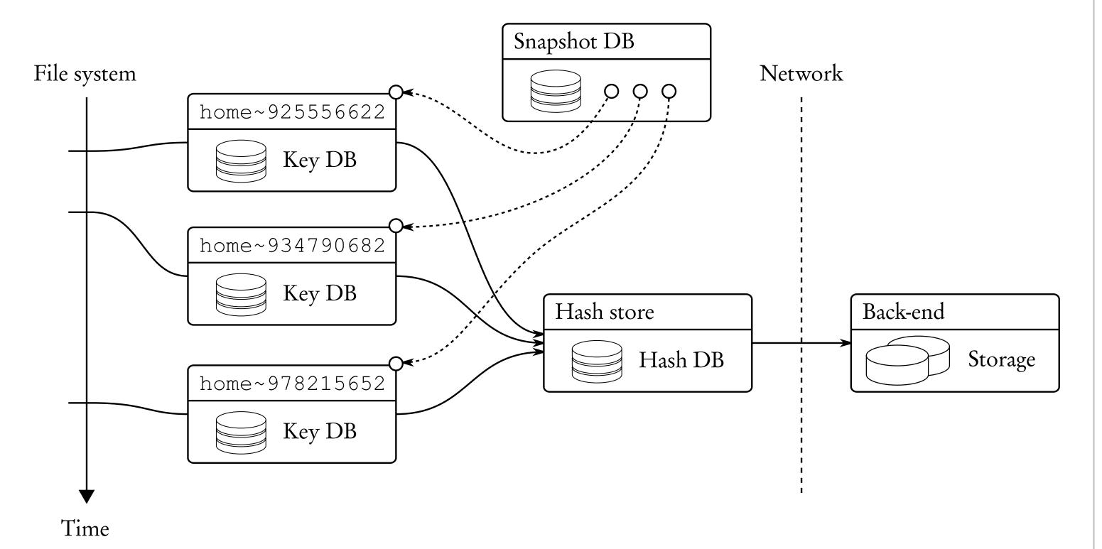
An overview of Hindsight. Each snapshot is represented by an database mapping file paths to data-blocks. The hash database knows where each file-block is located on the back-end. A snapshot database keeps track of all the snapshots. In this figure three snapshots named home was taken.
