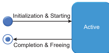
Figure 2.2: State transition diagram for nonblocking operations
