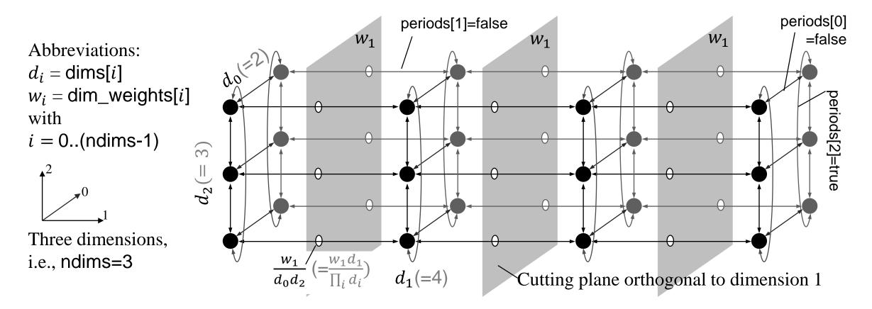
The arguments dim\_weights[i] i =0::(ndims-1), abbreviated with  $w_i$ , should be specified as the accumulated message size (in bytes) communicated in one communication step through each cutting plane orthogonal to dimension  $d_i$  and in each of the two directions.
