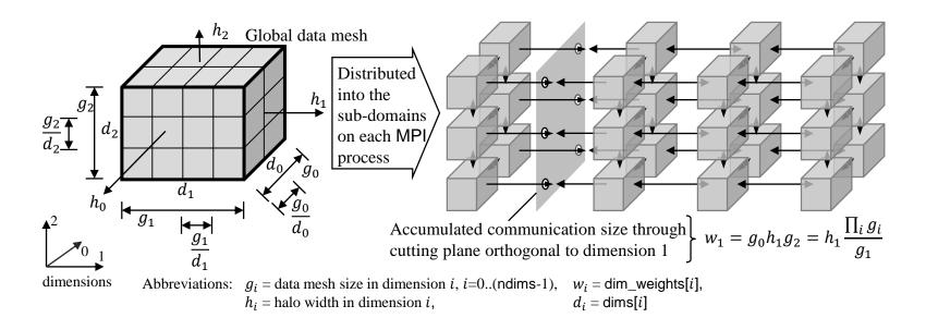
Example for the calculation of the accumulated communication size  $w_{i,i=0..2}$  in each dimension.
