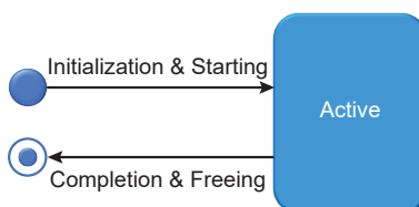
Figure 2.2: State Transition Diagram for Nonblocking Operations
