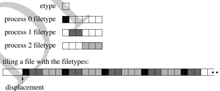
Figure 13.2: Partitioning a file among parallel processes
