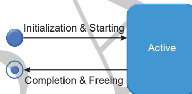
Figure 2.2: State Transition Diagram for Nonblocking Operations
