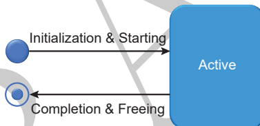
Figure 2.2: State Transition Diagram for Nonblocking Operations
