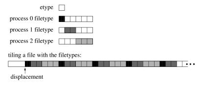
Figure 14.2: Partitioning a file among parallel MPI processes
