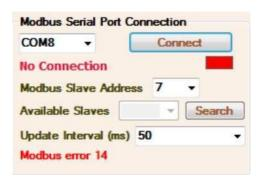
You may look in 'Devices and Printers' or 'Device Manager' for specific serial port of your device. The software supports serial ports up to COM32 only. If your device's port number is higher you can change it in - Device Manager > Ports (COM & LPT) > Double click on device name > Port Settings > Advanced > COM Port number
