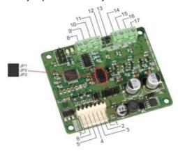
The three jumpers JP1, JP2 and JP3 can be set in the configuration as per the below table to provide a physical slave address to the drive. In the below table a value of '0' corresponds to a state where the jumper is not connected and a value of '1' corresponds to a state where the jumper is connected. If none of the jumpers are connected the drive has been programmed to use the Slave ID 11 in default mode which can be changed from 1 to 247 using GUI software or Modbus commands.
