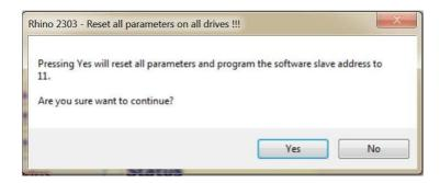
Click on "Yes" to reset the drive. After Clicking on 'Yes' if reset is successful confirmation message will be shown. Power off and Power on the drive to load default parameters. If any physical jumpers are preset at this point the slave id of the drive will be according to that otherwise slave id will be 11.
