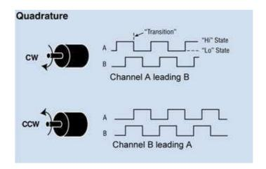
So drive can calculate the speed and direction of motor according to the pulses if number of Lines per Rotation is known. For each line drive gets 4 counts, for example if encoder is 334 lines drive can get 1336 (334  $\times$  4) counts per rotation. This parameter can be set in register 10. It's a 16 bit unsigned number having range of 1 to 65535.
