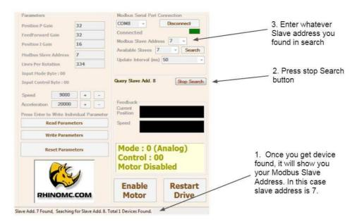
Make sure no multiple drives with same slave address is connected on serial bus.
