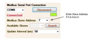
2. If slave address is not known or multiple drives with multiple addresses are connected on serial bus, click search button. This will search for all slave ids from 1 to 247. If any response is received from slave id it will give indication in status bar and list the drive in 'Available Slaves' drop down box.
