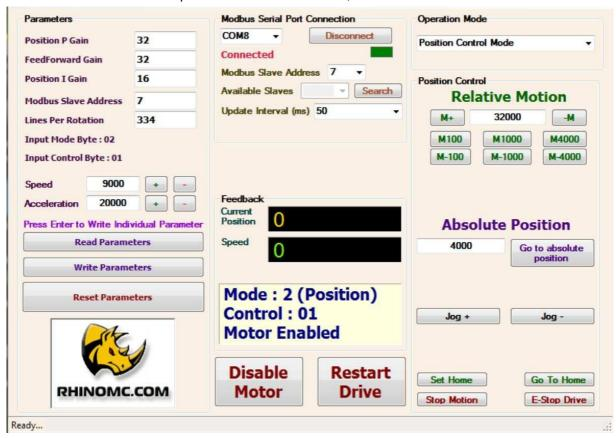
In Position control mode there are two ways to control position: **Absolute Position control** and **Relative Position control**.
