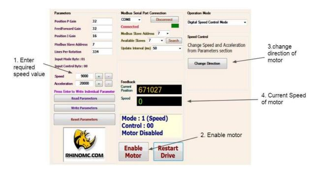
b) In this mode speed of motor(rpm) can be controlled by changing value from 0-65535.
