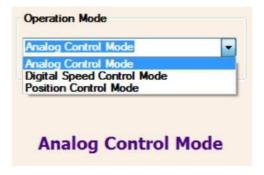
After selecting analog control mode click on "Write Parameters" to always start the drive in analog mode.
