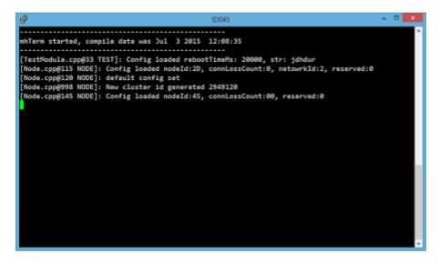
If you don't get output immediately it will sometimes help to disconnect the Devkit from USB for a short time or try to write something. This is an issue of the Segger Debugger chipset that bridges the UART.
