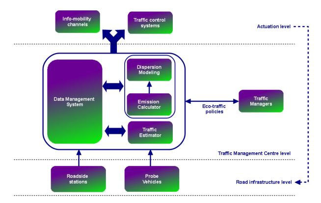
Figure 2: The simplified architecture of the INTEGREEN system.
