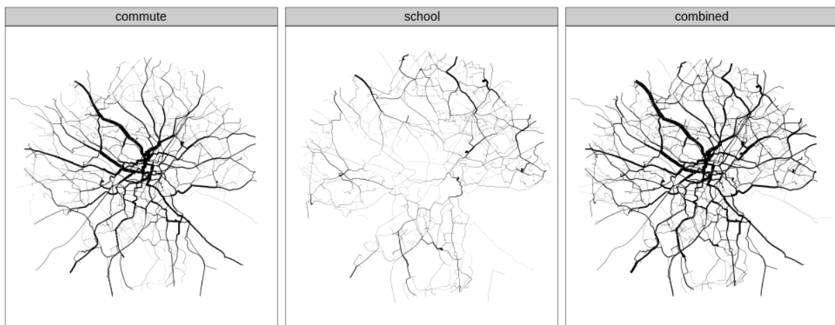
Figure 4: Route networks of commute, school and combined cycle propensity in the 5km zone surrounding Leeds Railway Station
