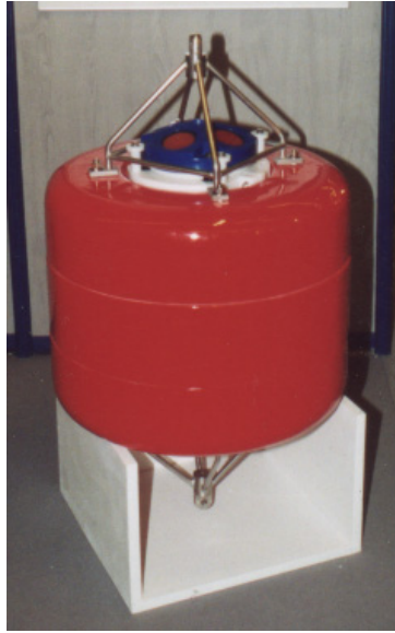
Figure 10. Subsurface Buoy Photo courtesy of Patrick Lefevre, Technicap. The Subsurface buoy was developed by BMTI and Technicap.
