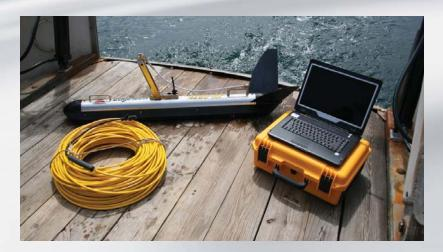
The 4200 Series is a versatile side scan sonar system that can be configured for almost any survey application from shallow to deep water operations. The 4200 utilizes EdgeTech's Full Spectrum® CHIRP technology to provide crisp, high resolution imagery at ranges 20-30% greater than non-CHIRP systems; thus allowing customers to cover larger areas and save money spent on costly surveys.
