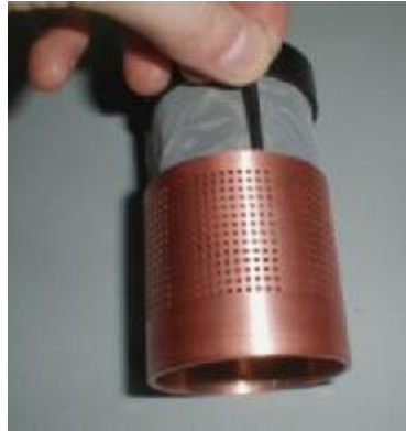
Figure F-5: Start positioning the copper screen
