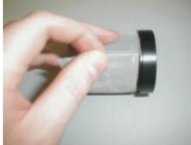
Figure F-3: Overlap the cloth over a groove
