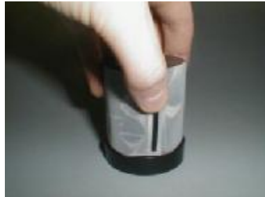
Figure F-4: Insert a plastic shim
