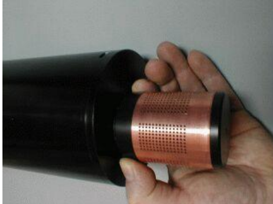
Figure F-9: Mounting the guard
