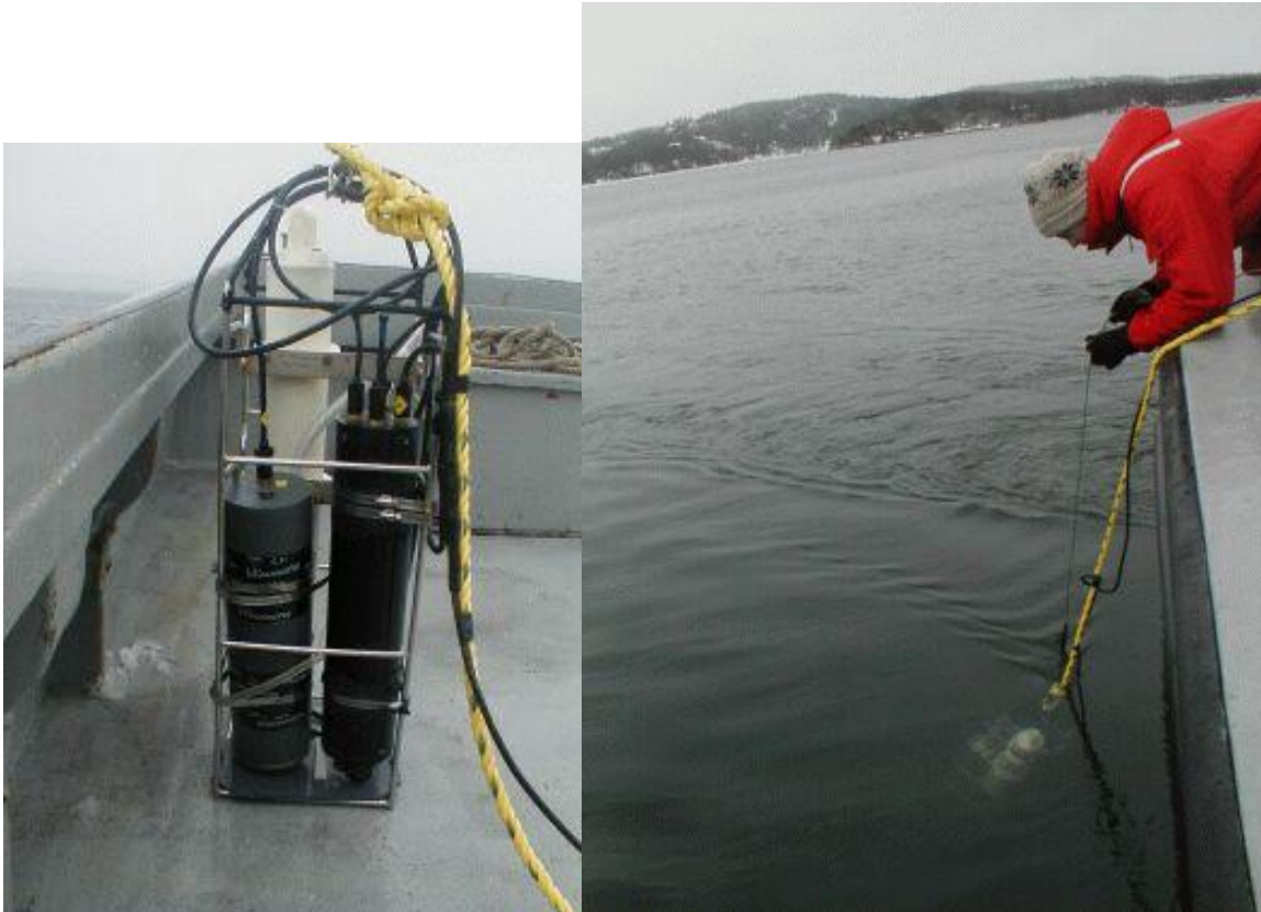
Figure C-3: CTD, ISUS, and Battery Pack
