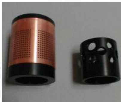
Figure A-13: Probe Guards
