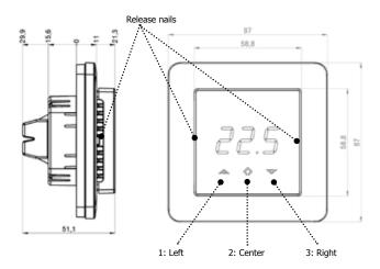
Use e.g. a small slotted screwdriver. Start by carefully removing the front cover by pushing the release nails. The front cover and the frame can now be removed.
