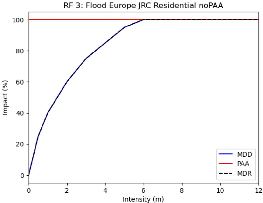
The plots illustrate how flood-depth is translated into a damage factor (0%-100%). The damage factor is then multiplied with the exposed asset in each grid cell to derive a local damage.
