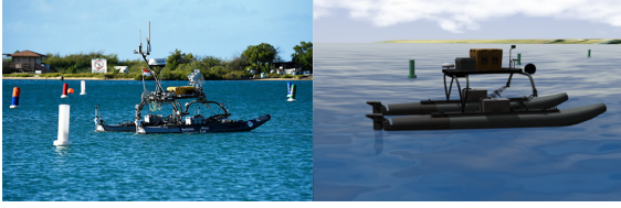
Fig. 4. A visual comparison of a physical WAM-V and course elements from RobotX 2018 (left) with a similar scene rendered in the VRX environment using Gazebo (right).
