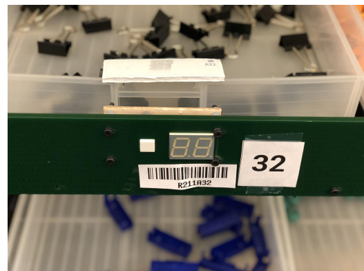
Figure 5. A source bin with identification methods. From top to bottom: a passive RFID, a two-digit seven-segment LED, a visual “32” and a printed barcode.
