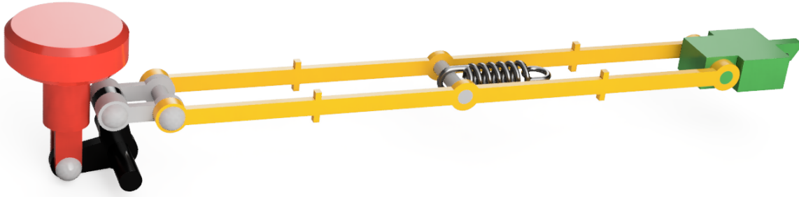
Figure 50 – Rendering of the latch mechanism. The parts are coloured to distinguish between them, in reality the only coloured part would be the button
