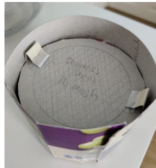
Figure 29 – Initial cardboard model of the filter cartridge with lid.
