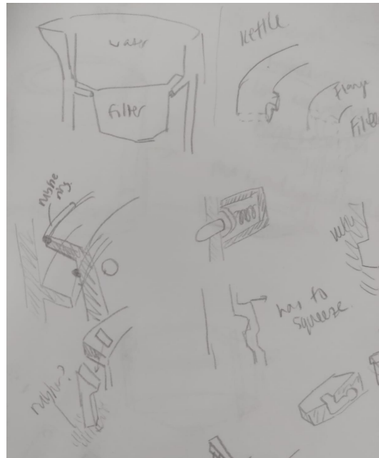
Figure 28 - Twist lock and push snap mechanisms considered for the filter lid. A spring resistive lock was eliminated as parts for this were intricate and many.
