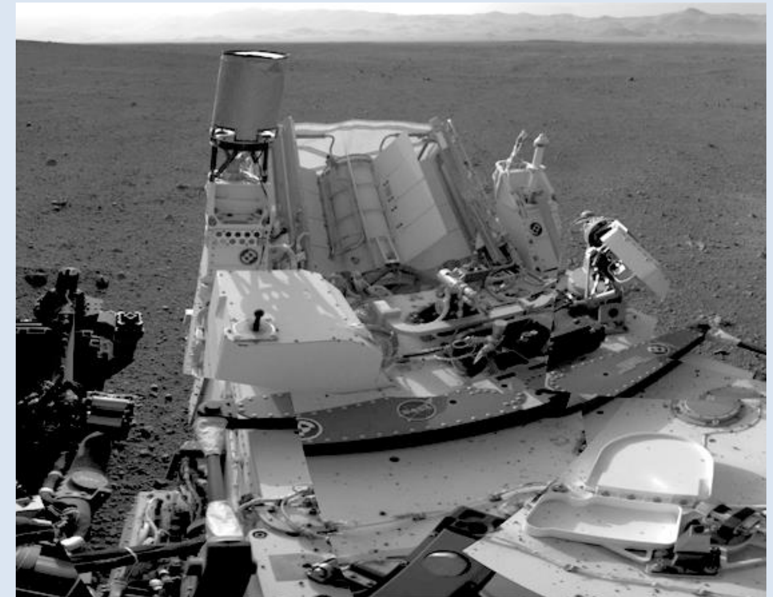
RTG installed in the Curiosity rover on the surface of Mars
