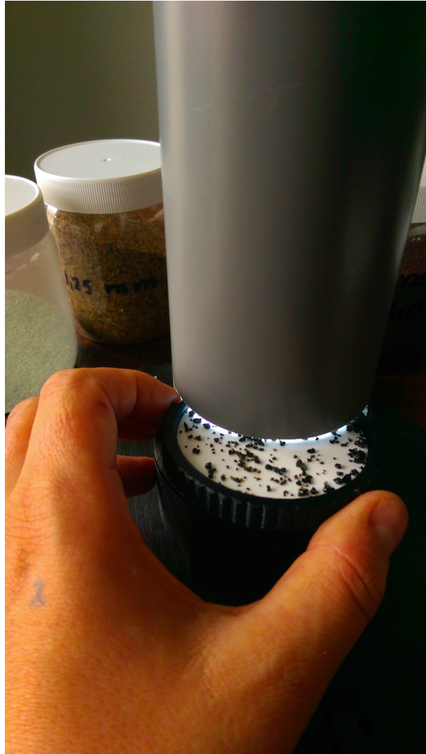
Figure 4.4: Placing the sample under the microscope
