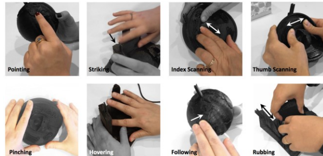
Figure 1. The eight gestures identified in the Elicitation section of the study. The movements of dynamic gestures are marked with arrows.
