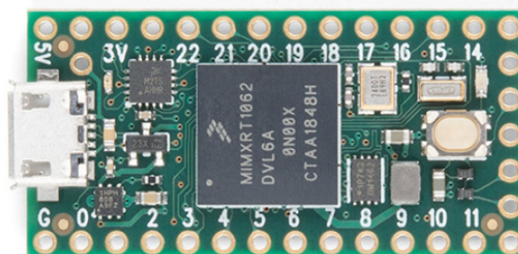
Figure 6 – Teensy 4.0, 0N00X mask
