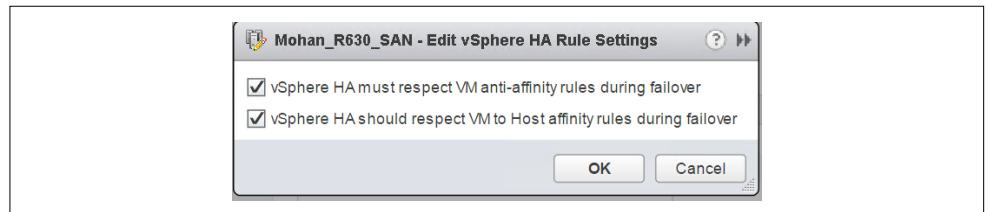
Figure 10: vSphere HA settings for anti-affinity for WSFC nodes set for a CAB configuration
