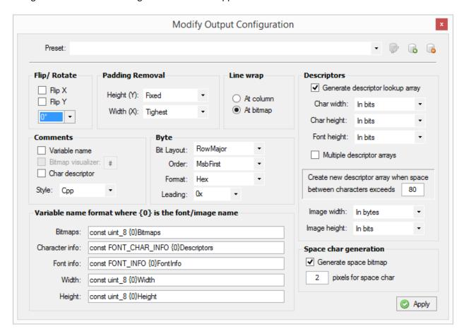
Once set, click **Apply** and then **Generate** to obtain the data in the Source file (.c) window. Right clicking on the window will allow the contents to be copied to the clipboard. It is highly recommend that this be copied to an editor as sections will be cut&paste into the fonts.cpp file.
