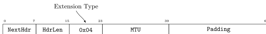
Figure 15.11: The header of the MTU extension. It is an end-to-end extension, thus the preceding NextHdr field has value 0xfd.
