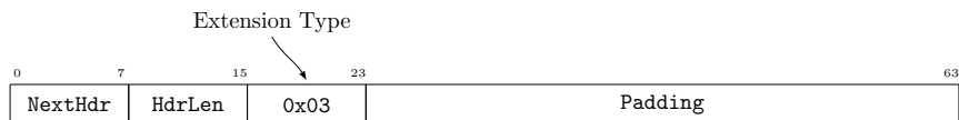
Figure 15.9: The header of the one-hop path extension. It is a hop-by-hop extension, thus the preceding NextHdr field has value 0x00.
