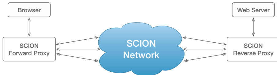
Figure 10.7: Deployment via SCION proxy.
