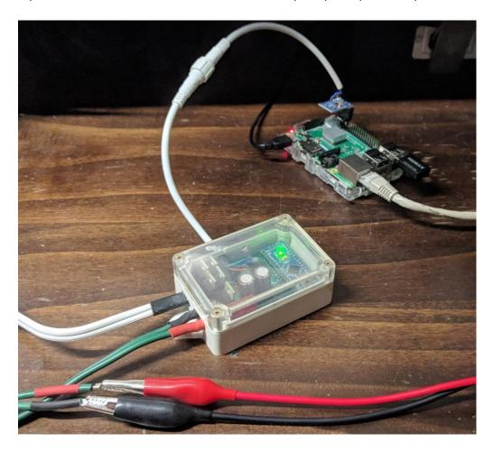
The Tx/Rx LED's on the Arduino should start flickering. Depicted is hardware purchased from the <a href="mailto:pypilot.org">pypilot.org</a> store. In case you produced the hardware yourself, remember that for a serial connection, Tx should be connected to Rx and vice versa.
