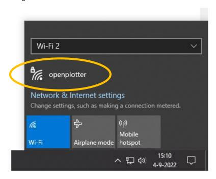
Note: if you have no internet connection to the raspberry (see later) the wifi connection might disconnect after a few seconds. Reconnect to it. You should get a 10.10.10.0 ip address.
