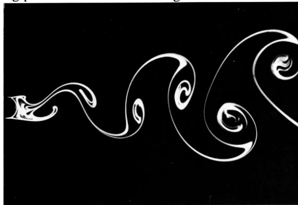
Figure 62. Kármán vortex Street with cylinder cross flow @ R=140 , V=1.4\text{cm/s} , \varnothing=1\text{cm} [75]
