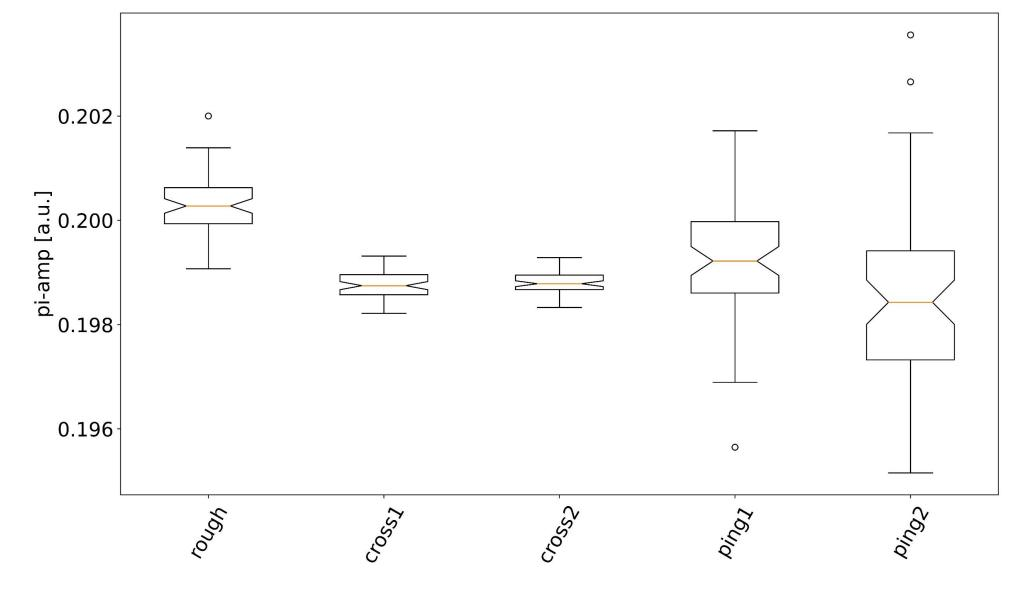
This plot shows the boxplot of the  $\pi$ -amplitudes of the rough, cross point (*cross1, cross2*) and ping-pong (*ping1, ping2*) calibration. The cross point calibration has a smaller variance, smaller range of the data (smaller whiskers) and no outliers.
