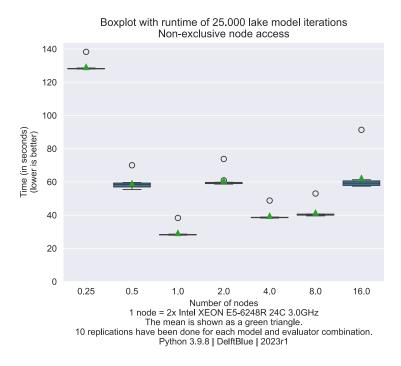
Notable is the almost linear performance scaling from 0.25 to 1 node, but the inconsistent scaling after that, without any system being faster than the 1 node one.
