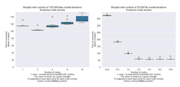
The lake model shows an performance improvement when running on two nodes, but nowhere near linear scaling. The flue model shows near-linear performance scaling from 0.25 to 2 nodes, but no significant scaling after that.
