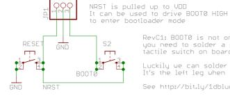
RevC1: B00T0 is not on the expansion header you need to solder a patch wire to the tactile switch on board
