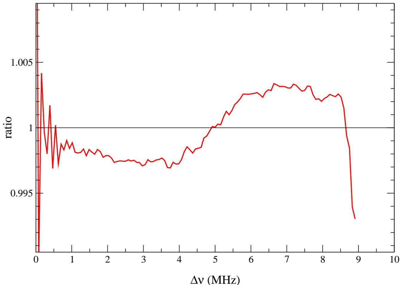
Figure 2: *Sum over all ifrs. The rapid variations on the left are the Gibbs ripple, i.e. an artifact of the FFT that produced the spectrum after correlation. The (antenna-based) IF's before the correlator have several filters. Temperature variations cause variations of different freq-scales. The large-scale variations seem to have the largest amplitudes in time (Kolmogorov-like?). This should be explained. The small-scale variations are partly noise.*
