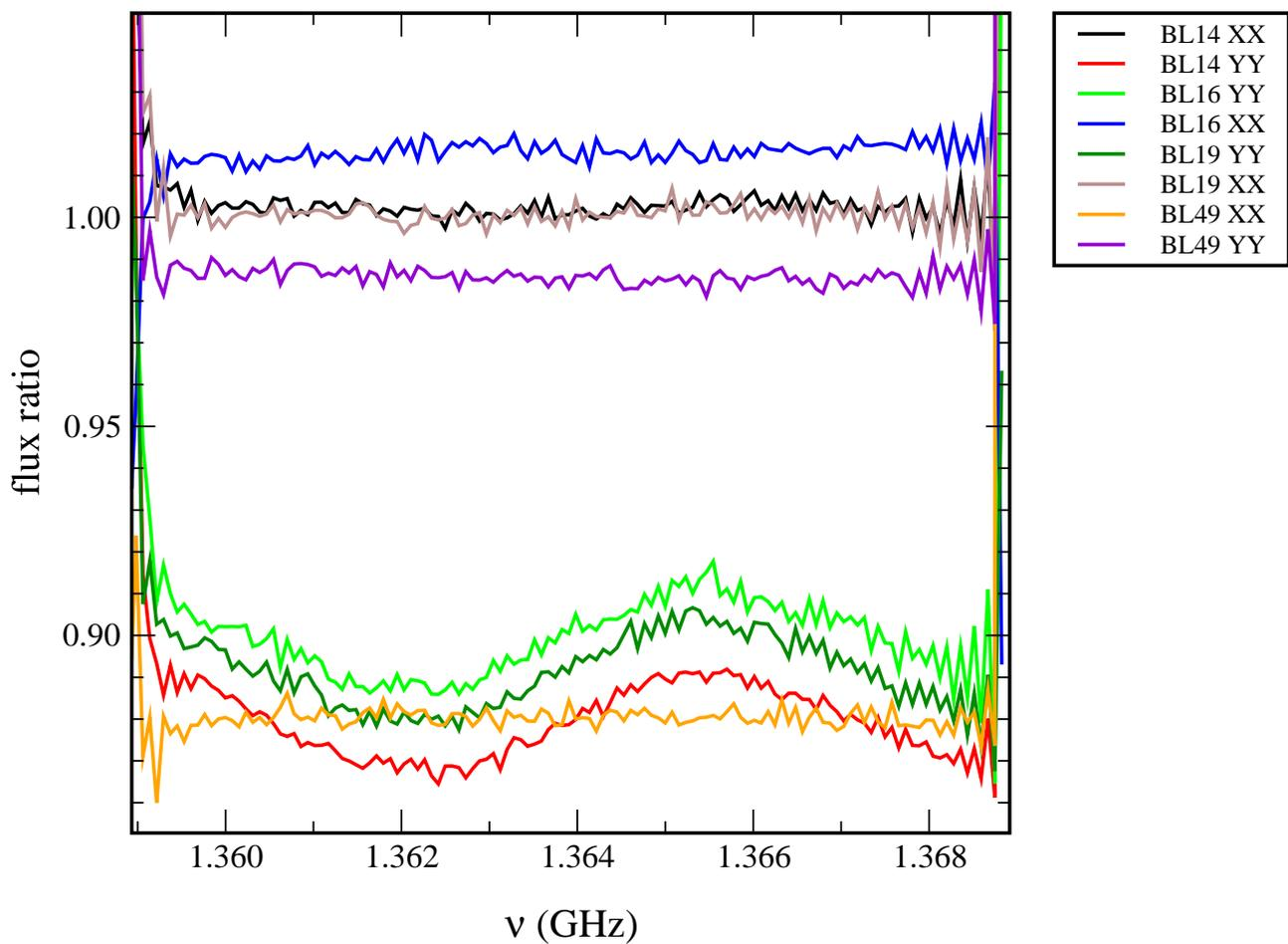
Figure 4: *Some ifrs have a stable bandpass, while others vary quite significantly in 12 hours. Note how the variation seems to be confined to the YY ifrs, and is remarkably similar even though different antennas are involved.*
