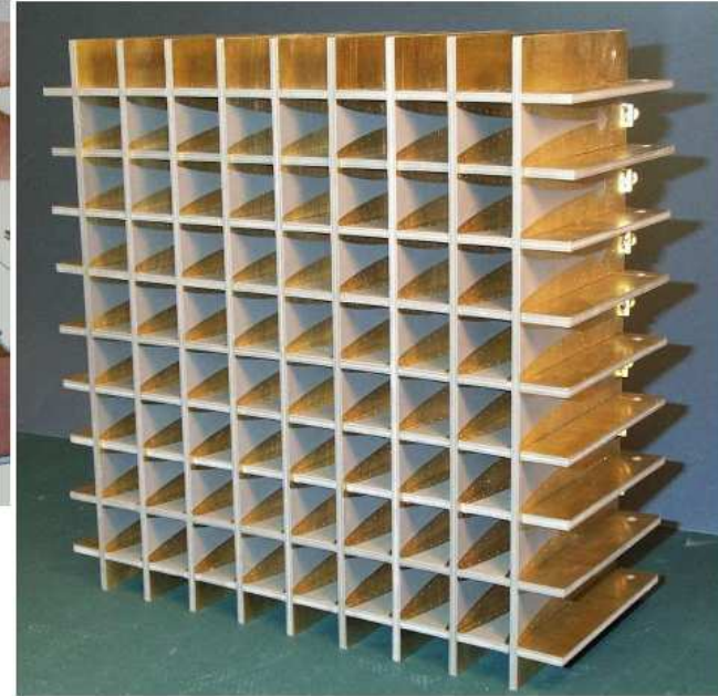
UMass Antenna Lab designed, fabricated and tested the above 8x9x2 array. Support was from ASTRON. Picture courtesy Dan Schaubert.
