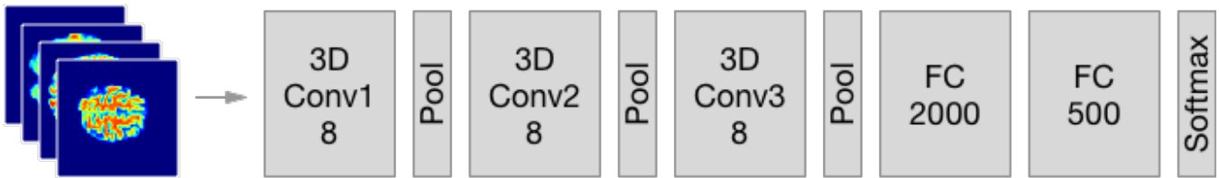
Fig. 2: The 3D convolutional network has 3 convolution layers, 3 max-pooling, and 2 fully connected layers, followed by a softmax output layer. All 3D convolution kernels are 3 \times 3 \times 3 with stride 1 in all three dimensions. Number of filters are denoted in each box. The 3D pooling layers are denoted as pool. All pooling kernels are 2 \times 2 \times 2 . The output units of the fully connected layers are denoted in each box.
