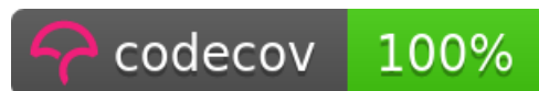
Fig. 2.11 A build badge for the code coverage of an R package ( https://github.com/ropensci/beautier ). The umbrella signals that the code coverage is hosted by CodeCov ( https://codecov.io/ ). The text indicates which process it is that the badge signals, which in this case, is that the code is fully covered by tests.
