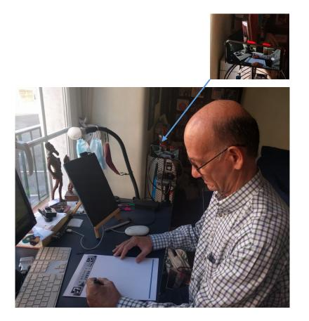
Acquiring a sequence of images from the camera (a video), the objective is to produce a sequence of output images with the sheet of paper corrected by the projective transformation between the table plane and the camera plane.
