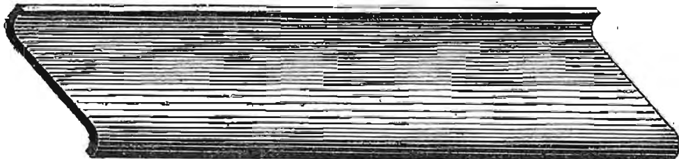
Girth 11".—16 Gauge up to \frac{1}{8} " thick, maximum length 6' 0". Under 16 Gauge, " " " 8' 0".
