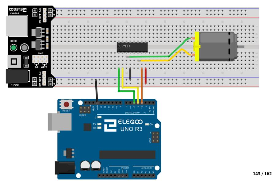
The code below does not use a separate power supply (ie a battery), it uses instead the 5v power from the Arduino. Note that this would be risky without the L293D controlling it.
