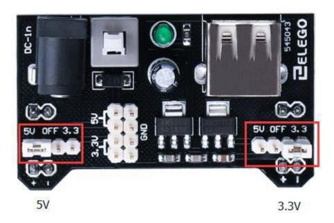
The left and right voltage output can be configured independently. To select the output voltage, move jumper to the corresponding pins. Note: power indicator LED and the breadboard power rails will not power on if both jumpers are in the "OFF" position.
