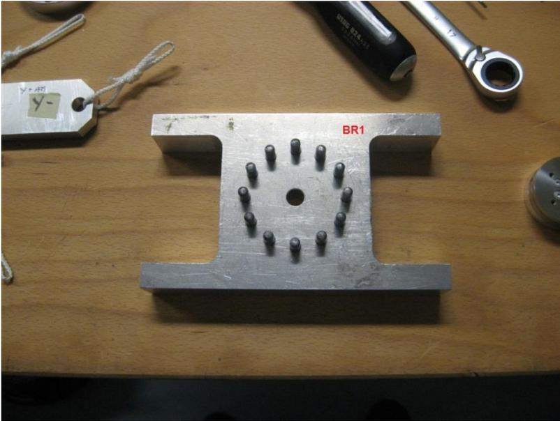
Figure 4: Custom made H bracket
