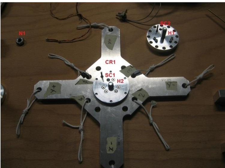
Figure 3: Custom made cross, heads and the nut
