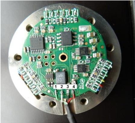
Figure 14: CAN and POWER cables soldered to the Strain PCB
