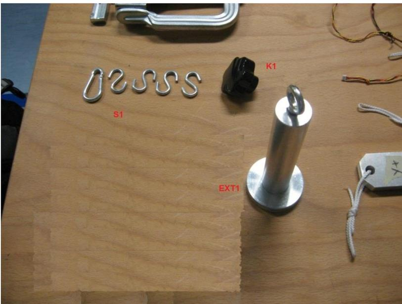
Figure 5: Custom made spacer, Z axis extension and knob
