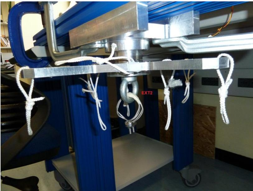
Figure 6: Custom made Z axis extension
