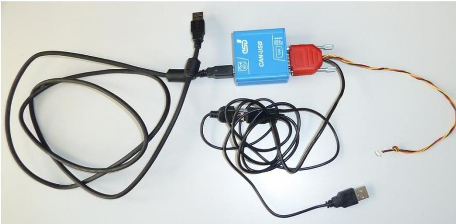
Figure 9: CAN-USB with its cables
