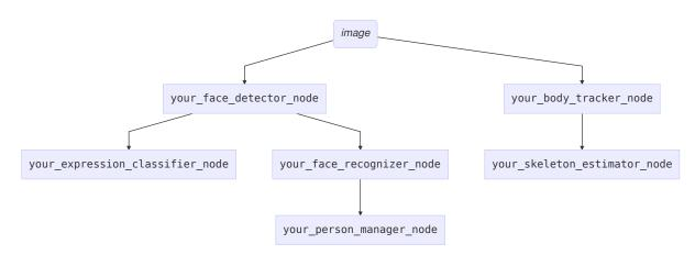
This possible pipeline is only for illustration purposes: depending on each specific pipeline implementations, some of these nodes might be merged or on the contrary, further divided into smaller nodes. For instance, one might choose to integrate together the face recogniser node and the person manager.
