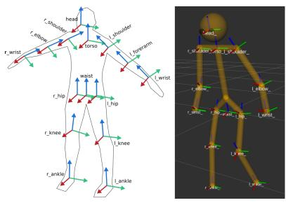
The main 15 links defined on the human body. Frames orientations and naming are based on REP-103 and REP-120. Right: render of the reference URDF model of the human body in *rviz*.
