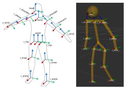
The main 15 links defined on the human body are presented in the above diagram. Frames orientations and naming are based on REP-103 and REP-120. Right: render of the reference URDF model of the human body in *rviz*.
