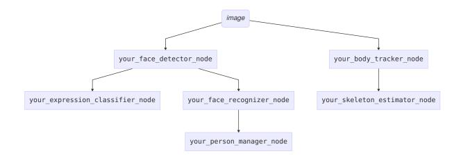
This possible pipeline is only for illustration purposes: depending on each specific pipeline implementations, some of these nodes might be merged or on the contrary, further divided into smaller nodes. For instance, one might choose to integrate together the face recogniser node and the person manager.
