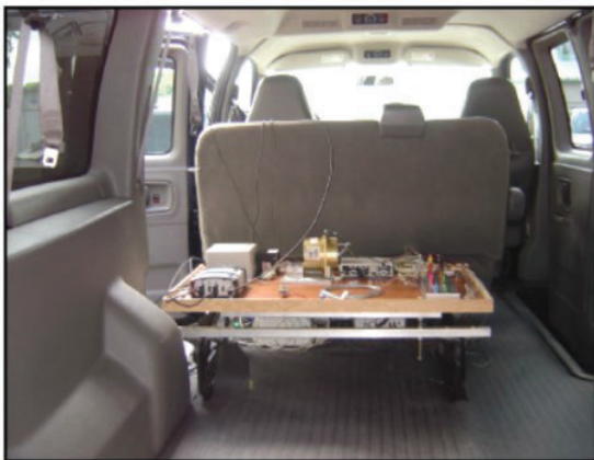
Fig. 3. Data logging equipment placed in a test van.
