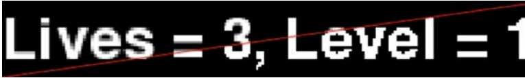
Figure 16-4. The anti-aliased version of the image is shown to the left of the red line
